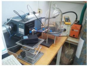
**Fig. 1b:** Photo of the experimental setup that shows the vacuum chamber, the pump, the power supply and the two spectrometers.
