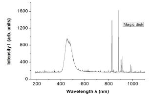
**Fig. 11:** The emission spectrum of the magic disk shown in Fig.9, observed with the Ocean Optics spectrometer.
