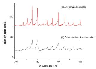
**Fig. 5:** Comparison of the emission spectrum of the second positive system of nitrogen (chamber pressure 15 torr) during an electrical discharge (dc voltage 3kV, 2.3 mA) observed with two spectrometers: (a) the AndorSR-303i -iDus, (b) the HR2000, Ocean Optics.
