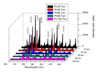
**Fig. 3:** Emission spectra of the second positive system of nitrogen at various pressures, during an electrical discharge (dc voltage 3kV, 2.3 mA) observed with the Andor303i-iDus420spectrometer.
