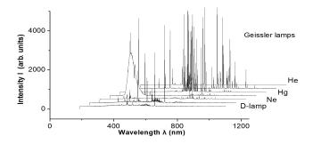
**Fig. 10:** Emission spectra of various gas discharge lamps (Geissler), during an electrical discharge (dc voltage 3kV, 0.5 mA) observed with the Ocean Optics spectrometer.
