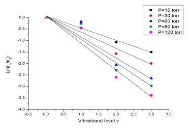
**Fig. 6:** Plot of the experimental values of  $\ln(n_v/n_0)$  as a function of the vibrational level v for 5 different chamber pressures. Spectra shown in figure 3 were used for the calculation of the populations  $n_v/n_0$ . Linear fitting of the data was used for the calculation of the slope and the estimation of the vibrational temperature from equation 4.
