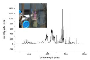
Fig. 2b: Emission spectrum of nitrogen  $N_2$  (chamber pressure 15 torr), during an electrical discharge (dc voltage 3kV, 2.3 mA), observed with the HR2000, Ocean Optics spectrometer. Photo shows the discharge light between the two electrodes.
