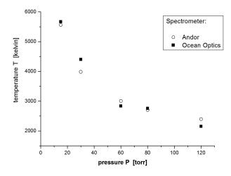
**Fig. 7: :** Plot of the experimental vibrational temperature as determined from figure 6 vs chamber pressure.
